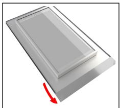
Fold down the soft flash that is tucked up at the bottom of the flashing tray.
