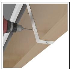
Fix locating straps to rafters/trusses using tech screws.
