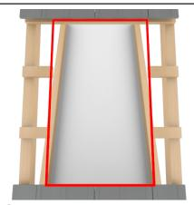
Cut tile battens (and rafter if required) and nog out as required.
