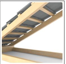
Decide location by inspecting inside roof cavity. Try to avoid obstructions such as hanging beams, under purlins, etc. whenever possible.
