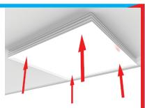
Plug driver into GPO then sit driver on top of light diffuser push light diffuser up and click into frame.
