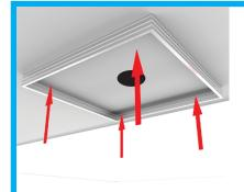
Unclip light diffuser from frame and mount frame to ceiling using fixings provided. Use existing hole to plug driver into GPO.
