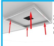
After a licenced electrican has installed GPO in your ceiling and switch to the wall unclip light diffuser from frame and mount frame to ceiling using fixings provided. Cut a 100mm square hole.
